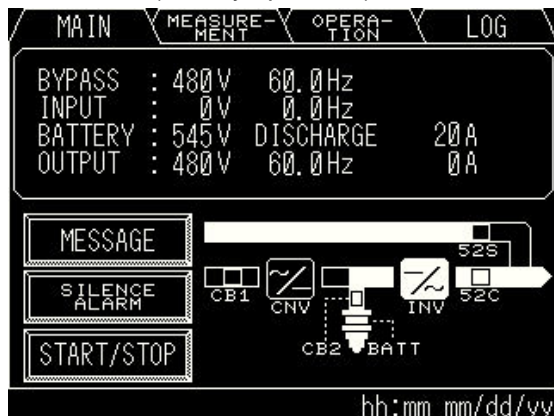
FIGURE 2.7.1 Main screen (Battery operation)
